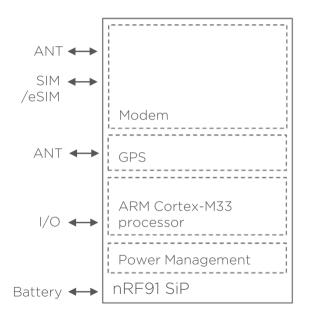
Support for cellular based positioning Modem support for Enhanced Cell ID and OTDOA
