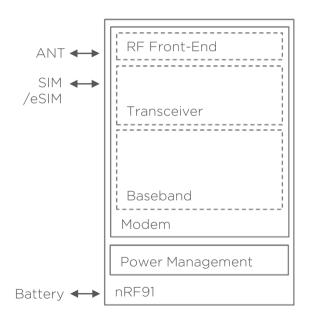
Complete modem in a package Multimode LTE-M / NB-IoT
